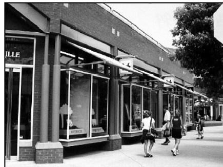
Figure 19: Ground floor levels of buildings in the CBD should encourage pedestrian activity with large windows, doors, and pedestrian scale details.
