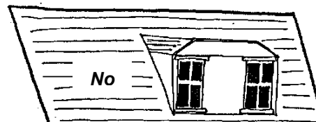
Figure 20: The roof on the top illustrates appropriate efforts to maintain the original dormer style. The roof on the bottom shows an inappropriate connection between the two original dormers to create a large shed dormer.
