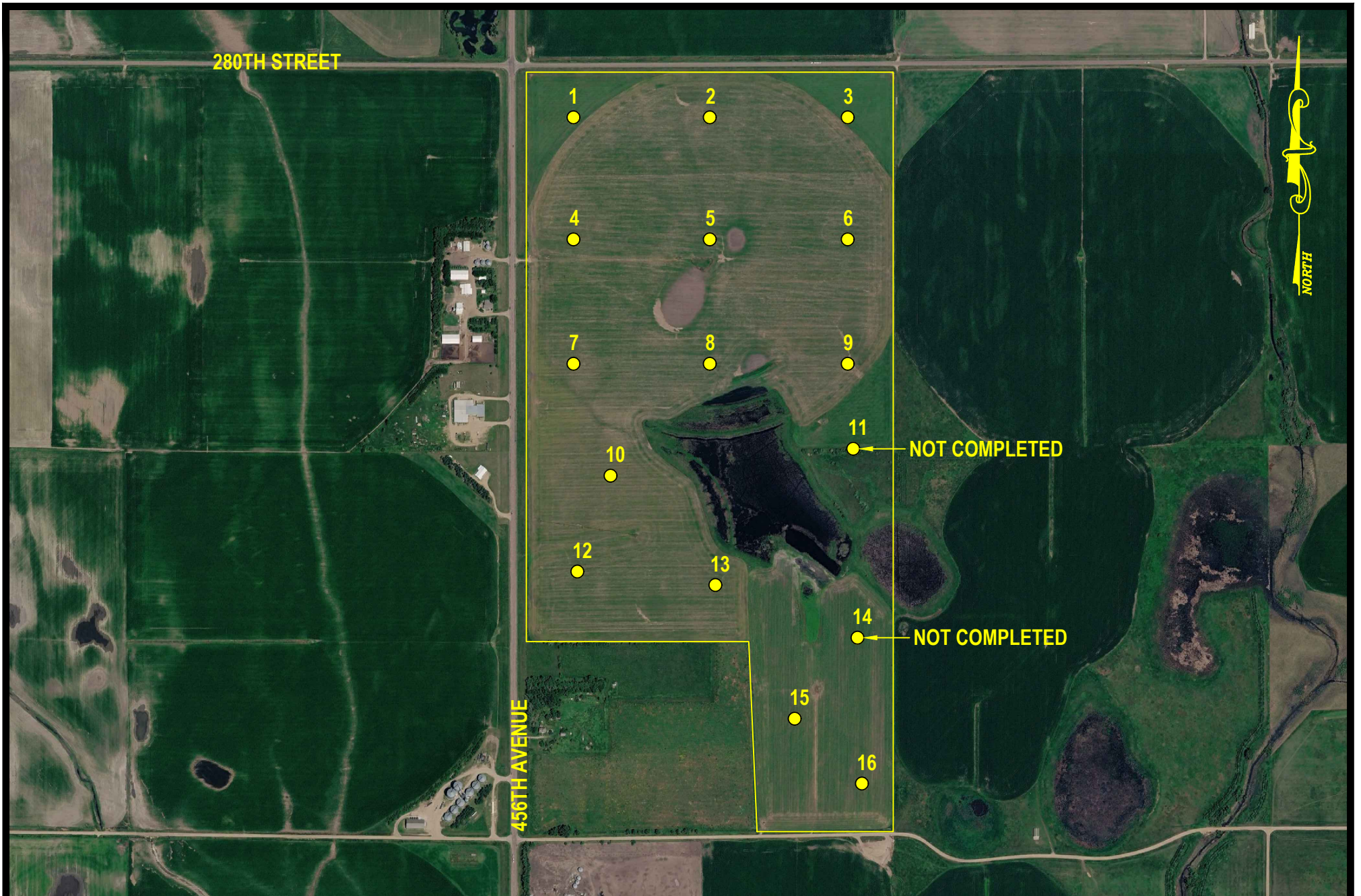
FIGURE 2 TEST BORING LOCATION MAP SAND & GRAVEL EXPLORATION 456TH AVENUE (S. OF 280TH STREET) NEAR PARKER, SD ACAD/GEOTEK/SHAWN/26-0686
