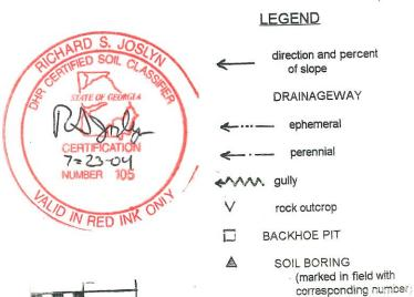
Soil boring locations illustrated on the soil map were located from existing corner pins and/or house-site stakes using compass bearing (Suunto KB-14) and paced distance.
